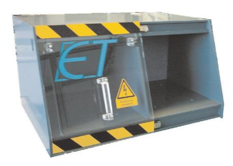
The standard basic dimensions, i.e., height (vertical-module grid) and depth (50 mm grid), of the tandem test hood HPH 4 can be optionally modified.
